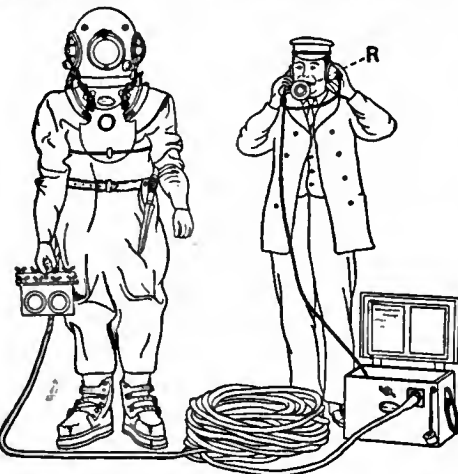
FIG. 4.—Diver's Telephone Communication with the Surface.
